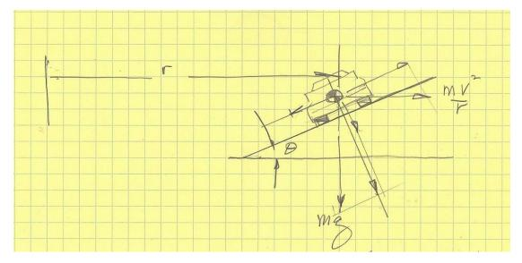
The extra variable  $\theta$  changes the equation to v = (((32.17\*r(0.8\*cos  $\theta$ +sin  $\theta$ ))/(cos  $\theta$ -0.8\*sin  $\theta$ )))^(0.5) where 32.17 is the gravitational constant and 0.8 is the coefficient of friction.
