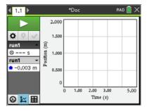
3. Press **Tab** until the **Start Collection** button is highlighted. One person holds the CBR 2 while another person holds the ball at least 15 centimeters beneath the CBR 2. Start the data collection by pressing Enter just before dropping the ball. You want the CBR 2 to record the initial height of the ball as well as the bounce heights.
