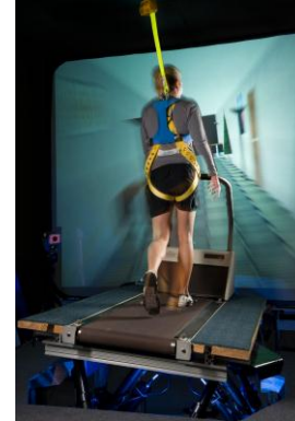
Figure 2: Test subject on the motion base treadmill
