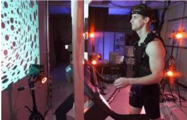
Figure 1: An instrumented test subject walks on a treadmill while viewing a rotating visual flow
