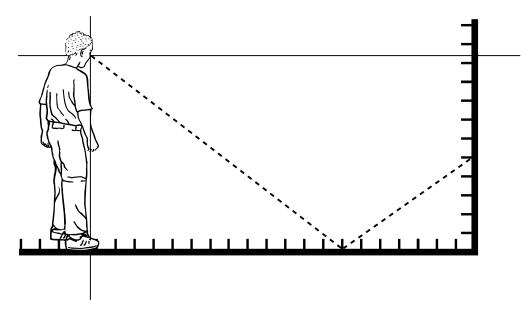
7. Ask the spotter to walk slowly towards the paper strip on the wall until the reflection of the numeral 20 can be seen in the mirror. Mark the position of the spotter's toe on the paper strip on the floor. Record this position in the table on the **Data Collection and Analysis** page.
