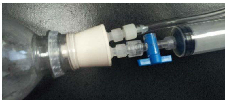
Figure 2: Bottle with pressure/fill cap
