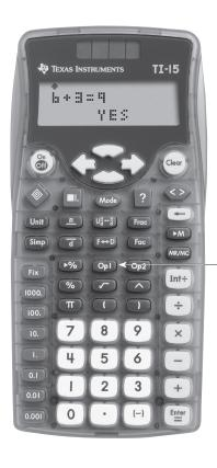
To define an operation (formula) first press the Op1 (or Op2) key then type the steps of the operation and then press Op1 (or Op2) to set the operation
