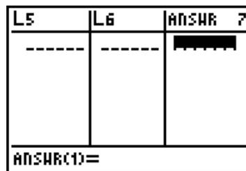
7. Enter "A". Press  $\text{2nd}$  [TEXT]. Move the cursor to each character of the entry "A" and press  $\text{ENTER}$ .
