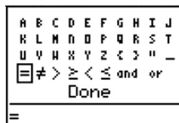
14. Press  $\downarrow$  [ENTER] to exit the Text editor and paste the equal sign next to L1.
