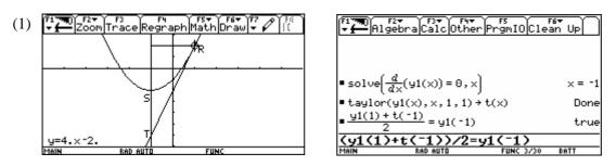
Note:First screen:The equation of the tangent line is found by using a graphic tool (F5).Second screen:The equation of the tangent line is found by using a CAS tool (Taylor polynomial of degree 1).
