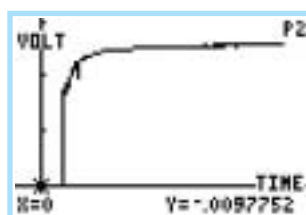
Graph showing the rise in voltage across a bulb as it is switched on.
