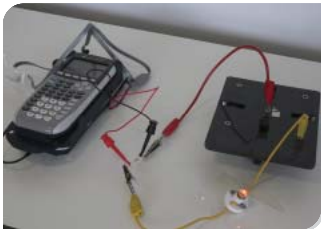
Circuit and probe leads connected across the resistor
