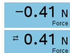
Press **[menu]** then choose Set Up Sensors ► Reverse from the
