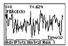
The force will look very uneven because the range on the y-axis is very small. As long as you pull with a constant force, your results should be fine. If your graph has any spikes or dips that are much larger than the rest, select  $\widehat{\text{Main}}$  to return to the Main screen and repeat steps 5 and 6.
