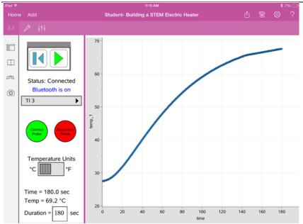
Possible results from project evaluation. The data shown was from a straw with 80 turns and was allowed to heat for 4 minutes, 30 seconds.
