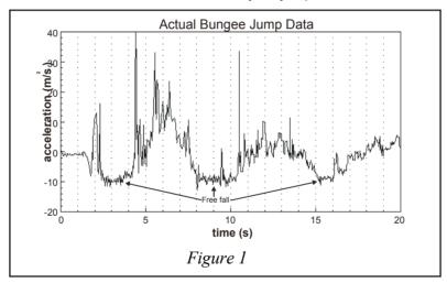
In your experiment, a block of wood or a toy doll will substitute for the jumper, and a rubber band will substitute for the bungee cord. An Accelerometer connected to the "jumper" will be used to monitor the accelerations.
