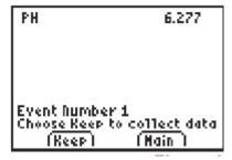
7. Insert the probe into the second sample and wait for the reading to become stable. Select **Keep** to collect the pH reading. Continue for a total of 8 trials (or the number of samples you have). With each recorded value, a new data point will be displayed on the graph with the option to **Keep** or **Stop** the data collection. The **Selected Events** feature will keep track of which reading you are on, increasing it by one each time you select **Keep**.
