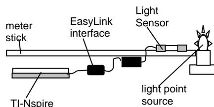
**Step 2:** Students should move to page 1.3, which contains an empty *Lists & Spreadsheet* application, and insert a data collection box. They should then connect the EasyLink or Go!Link to their handheld or computer. Tell students which setting (0-600, 0-6000, or 0-150,000 lux) on the Light Sensor to use.
