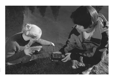
b. When the reading has stabilized, select START to begin sampling. **Important:** Leave the probe tip submerged while data is being collected for the next 10 seconds.
